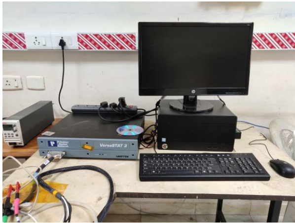
Versastat 3 electrochemical work station with EIS setup.
