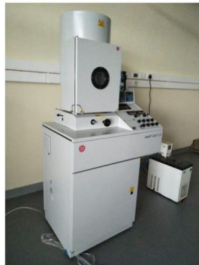
HHV Dual source thermal evaporator for solar cell fabrication (BRNS funded; ~ Rs 13 lakhs)
