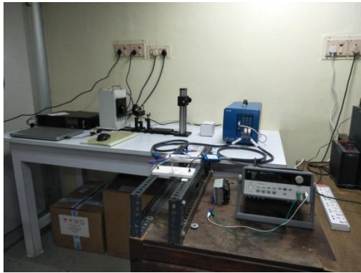
Photoelectrochemical workstation (home made) for solar fuel studies.
