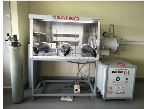
Hydropneovac Inert atmosphere glove box for solar cell fabrication (IIT Madras funded; ~ Rs 10 lakhs)
