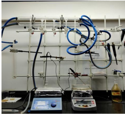
Schlenk line for air free chemical synthesis
