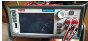
Keithley sourcemeter for electrochemical deposition of films (3 Nos)
