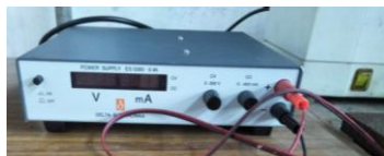
Delta Electronika high voltage DC power supply for electrophoretic deposition
