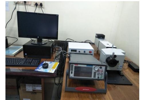
Spectroelectrochemical work station (home made) and external quantum efficiency analyser for solar cell and solar fuel systems characterization.
