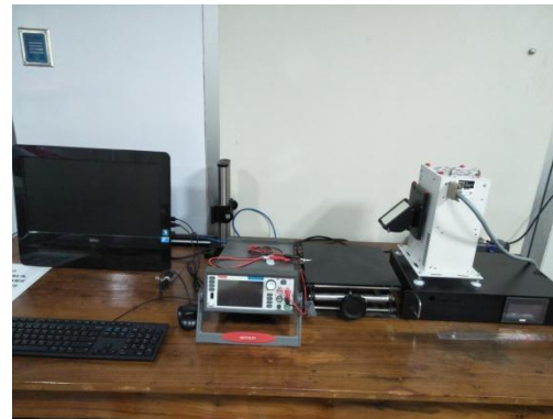
Photovoltaic station (home made) for solar cell characterization.
