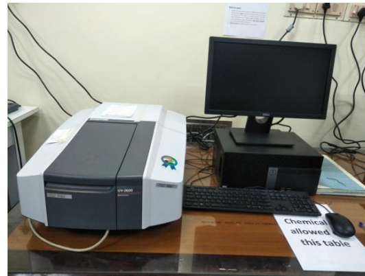
Shimadzu UV-Vis-NIR (190 nm to 1400 nm) spectrophotometer fitted with integrating sphere for solids, films and powders.
